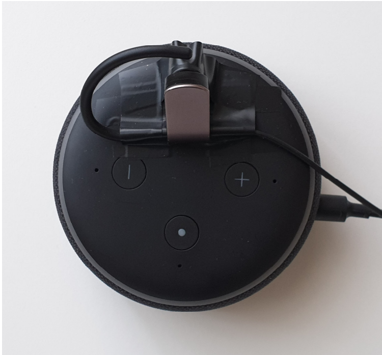
Figure 22: Alexa prototype - Echo Dot with Bluetooth headphones
