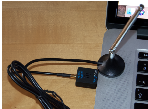
Figure 3.2.: NooElec NESDR Nano 2+ with MCX antenna plugged into a MacBook Pro mid-2014 model.
