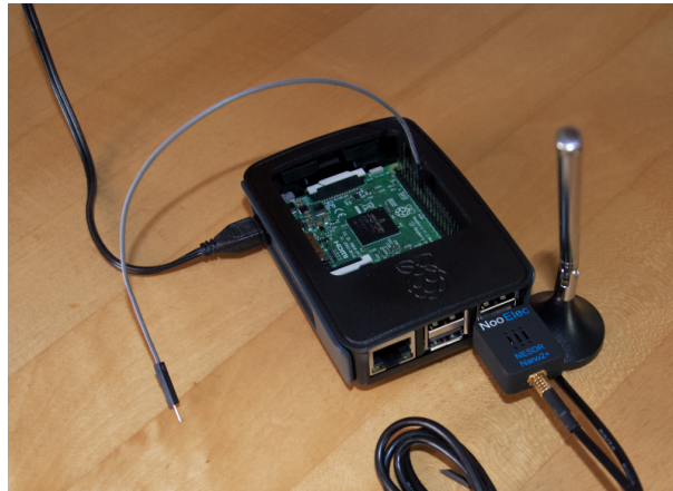
Figure 3.14.: Raspberry Pi 3 Model B with a male-to-female jumper wire connected to GPIO pin 18 as antenna and the NooElec NESDR Nano 2+ plugged into one of its USB ports.
