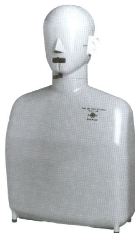
Figure 2.16 HATS for acoustical research [BEG00]
