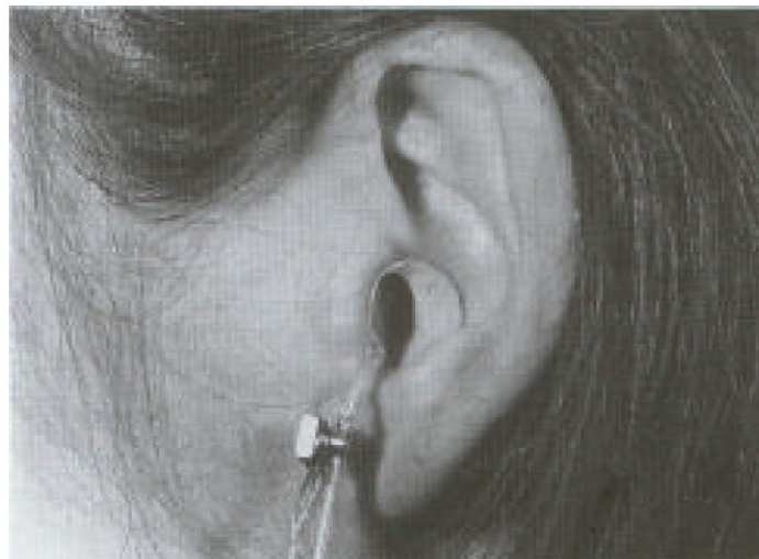
Figure 2.12 Placement of the microphone [WK89a]
