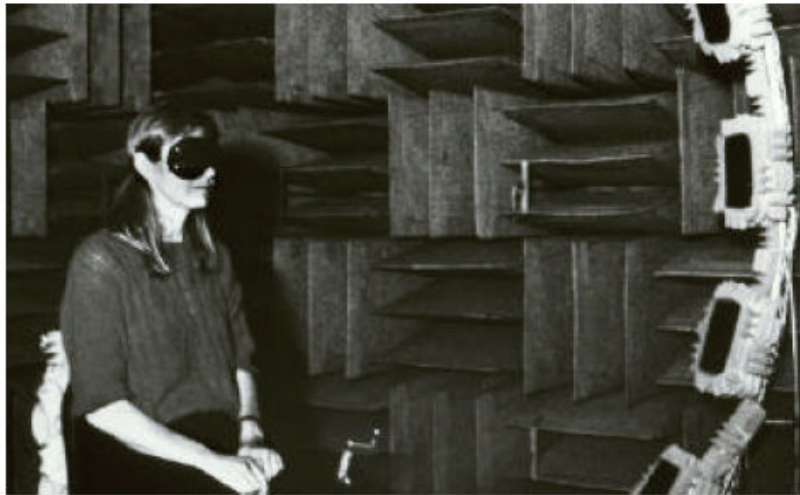
Figure 2.13 A subject in an anechoic chamber with the movable arc [WK89a]
