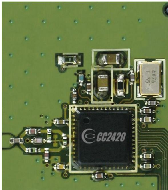
Abbildung 4.8: Transceiver-Chip: CC2420 [15]
