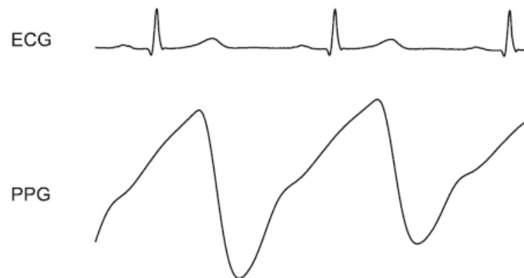
Figure 7 AC component of PPG and corresponding ECG (Allen, 2007)
