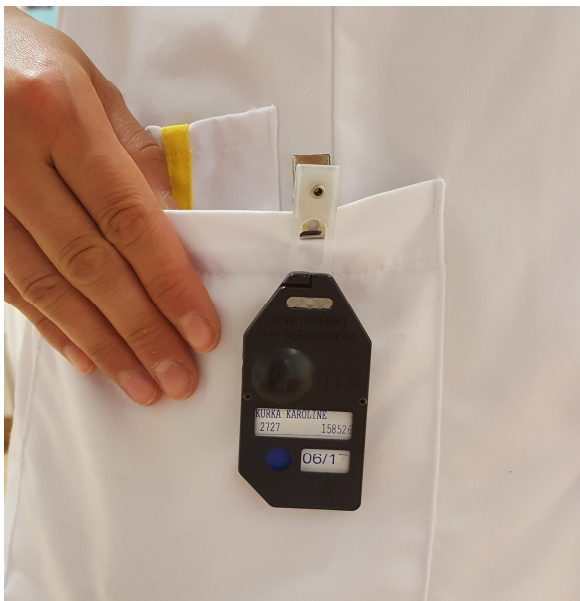
Figure 2: Correctly worn dosimeter mounted on the workwear in hip height.
