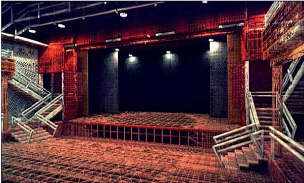
Abb. V-48 | Radiosity Rechengitter
