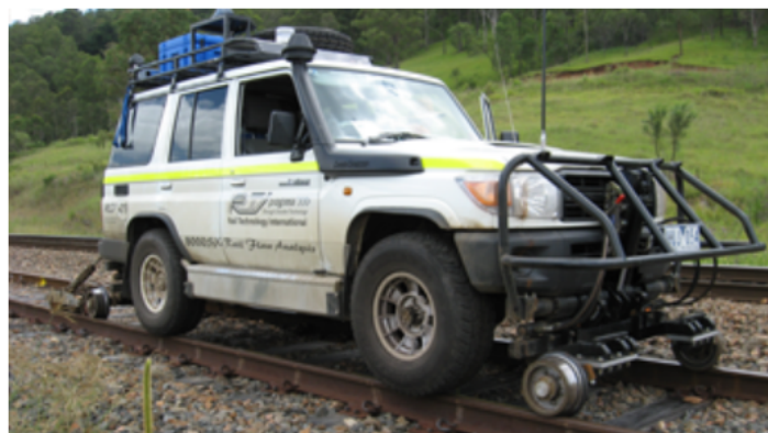
Figure 10: RRV with ultrasonic measuring equipment
