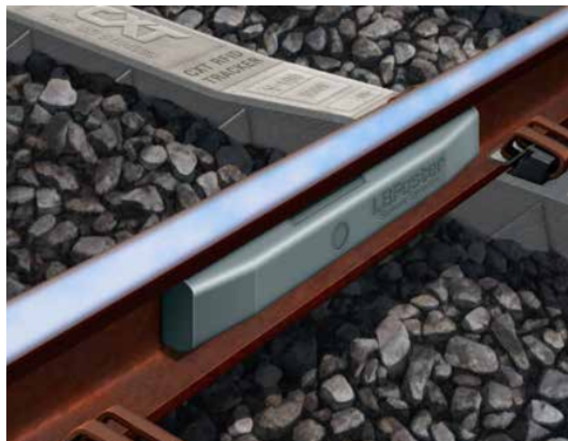
Figure 5: Measuring unit based on strain gauges [17]
