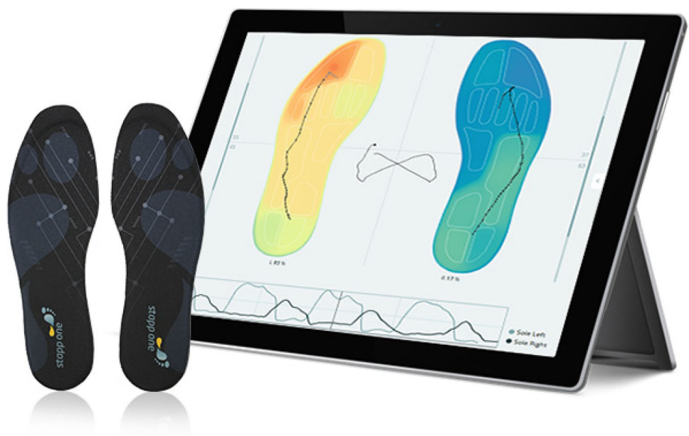
Fig. 2 Insoles and graphical user interface of the PC software used with them showing the pressure map for both insoles and the path of the center of pressure during a step
