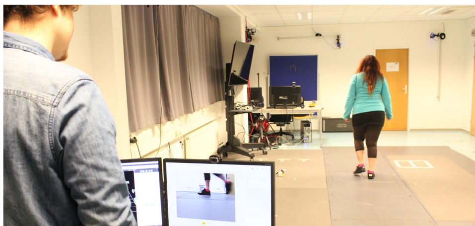
Fig. 3 Parallel recording of force plate and insole data with additional motion tracking
