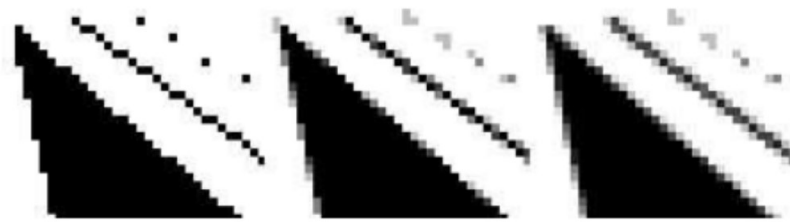
Figure 2.12. Three different levels of anti-aliasing. Left: One sample per pixel, middle: four samples per pixel, right: eight samples per pixel. (in a grid pattern)
